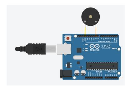
2. Using the circuit created in point 1, create a program that plays the notes Dó, Ré, Mi, Fá e Sol through the buzzer.
