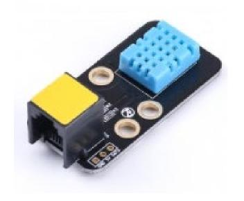
Temperature and Humidity Sensor Module
